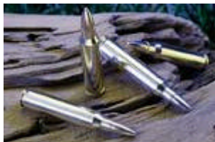
PolyOne’s nylon 12 filled with 96% tungsten is being tested as an environmentally safer replacement for lead in the U.S. Army’s “green ammo” program.
